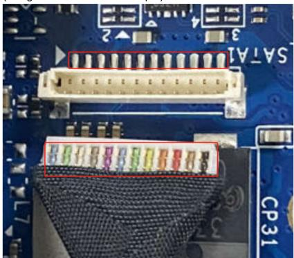
Insert the connector vertically and apply gentle downward pressure on both sides simultaneously (taking care not to shake it).
