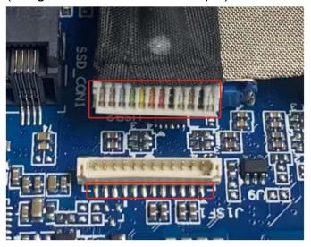
Insert the connector vertically and apply gentle downward pressure on both sides simultaneously (taking care not to shake it).
