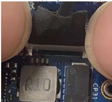
The side of the SATA cable with a colored stripe should align with the 12-pin connector on the motherboard, as shown in the red box in the diagram below (using P1/U56/U58 as an example).
